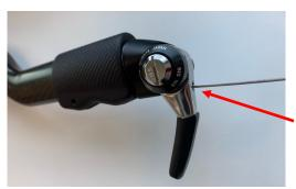
Now that you know the inner cable runs smoothly through the outer cable, attach the lever and pin to the body
