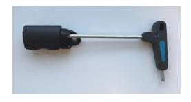
Take your shifter body and screw onto the expander bolt
