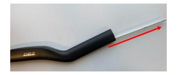
Take your outer shifter cable and run it through the bottom of the pole so that it pokes out the top
