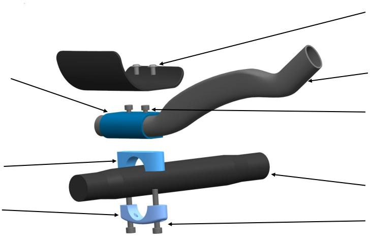
M5 x 8mm Button head screws (x4) (torque to 4nM)
