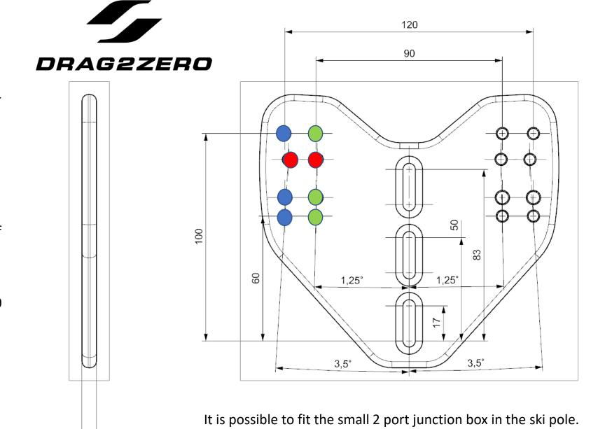
It is possible to fit the small 2 port junction box in the ski pole. The 3 and 5 port versions can be mounted on the plate using a cable tie.
