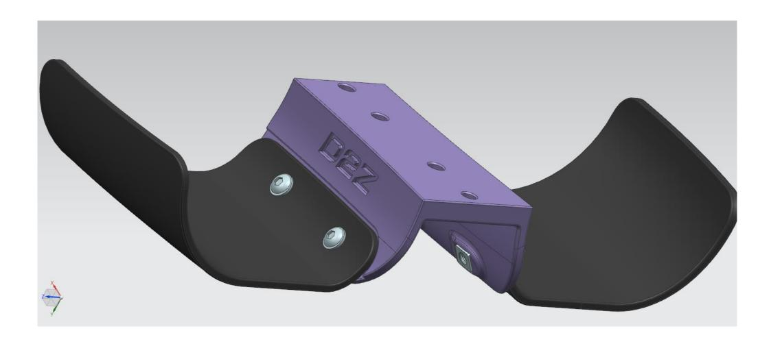
**Step 3**: Place bottle cage on top by aligning the holes of the cage with the holes in the mount
