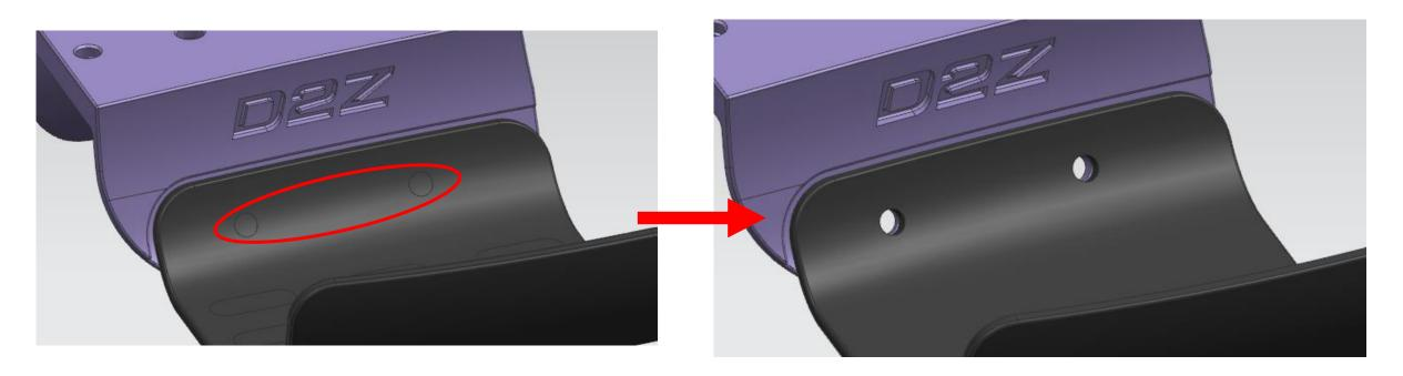
Step 2: Insert M5 flanged screws into armrests
