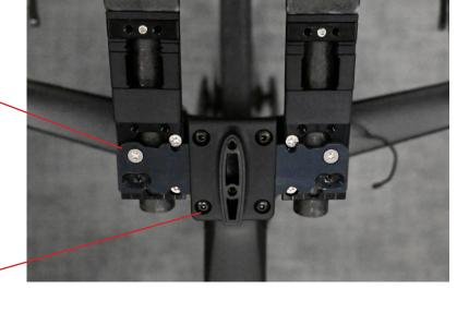
Mount on the outer set of holes as shown bellow.
