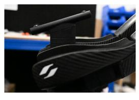
Step 10 Mount your bottle cage to the BTA bottle cage rail. Tighten to 2Nm
