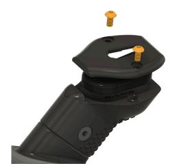
1. Loosen 2 M3 button head bolts and place SRAM Wireless AXS blip into grip
