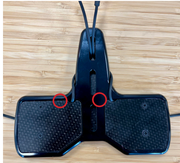
Under Panel Routing
